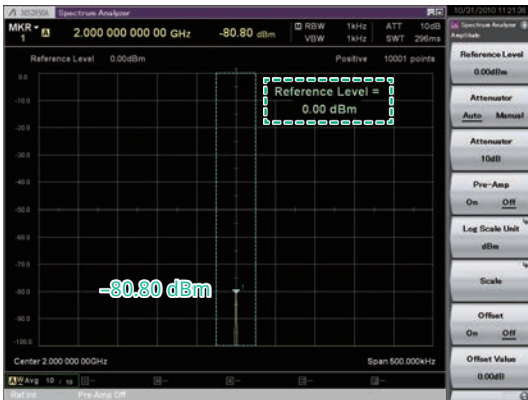
Example: Level Stability by Switching Reference Level
