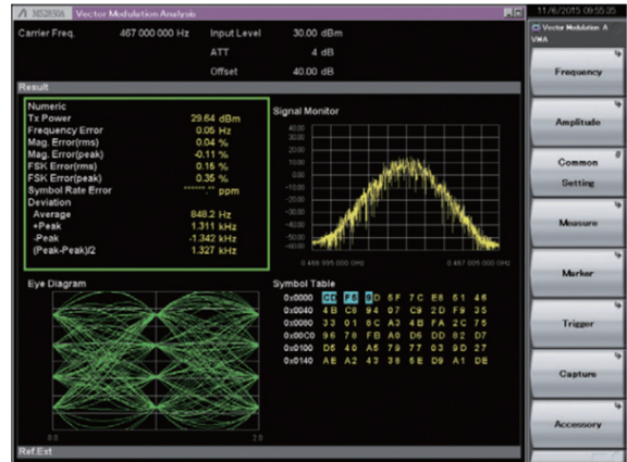
4FSK Modulation Analysis Measurement Example
